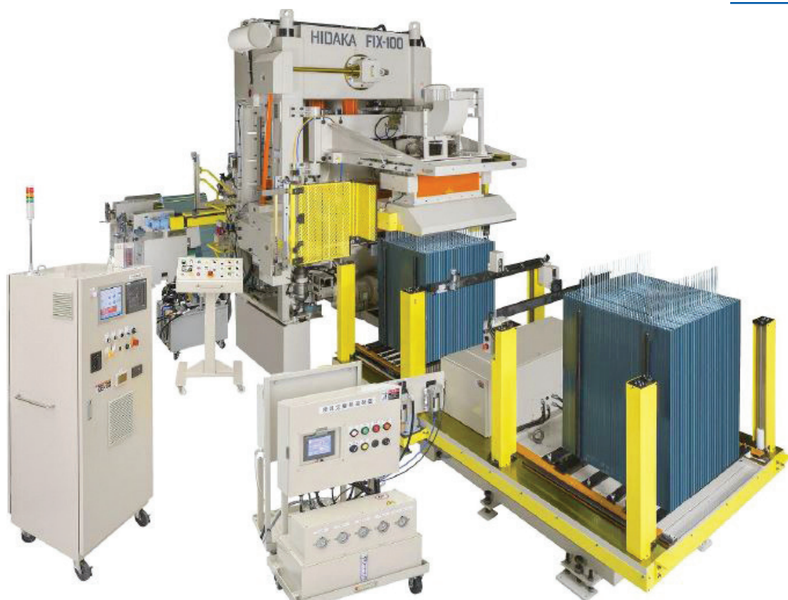
A Hidaka-make Fin Press - 7mm installed at Blue Star's Himachal Pradesh Plant
