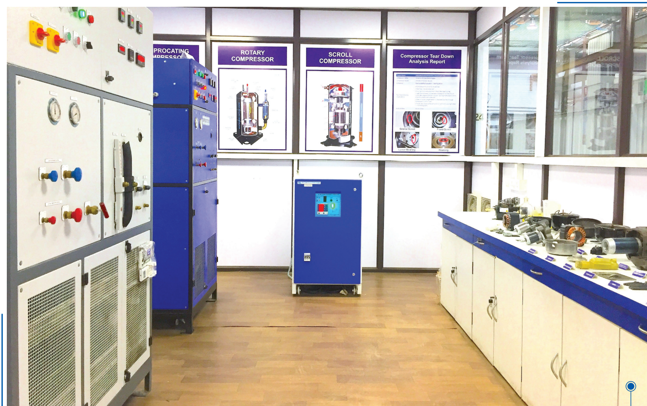
Compressor Lab comprising two Compressor Test Rigs and Cut Sections of Tested Compressors at Blue Star's R&D facility in Thane
