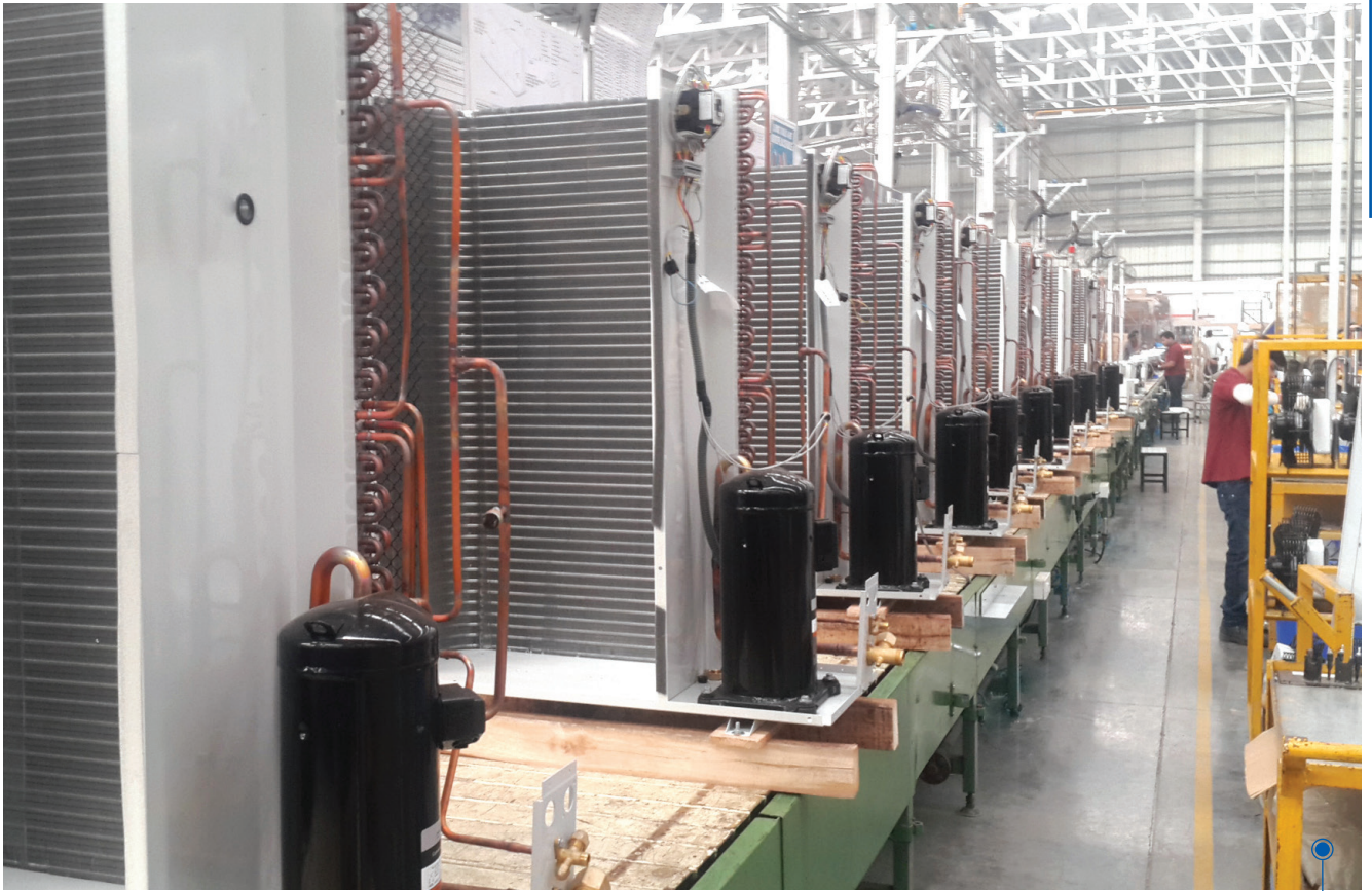
Refrigeration condensing units being produced at Blue Star's Wada Plant
