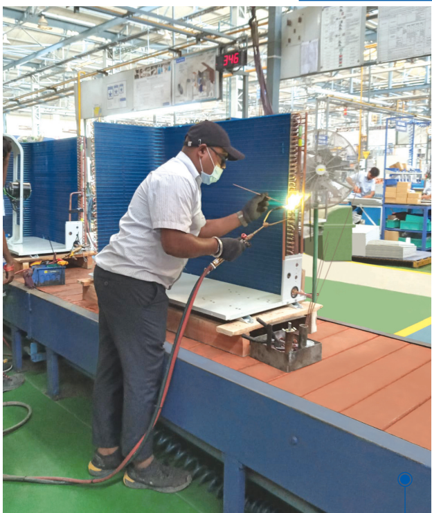
Manufacturing of ducted outdoor unit at Blue Star's Dadra Plant
